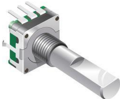
Rotary encoder (continuous rotation, produces 24 pulse per revolution in quadrature outputs)
