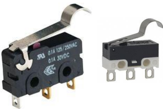
Microswitch and sub-microswitch are Single-pole Double Throw (SPDT)
