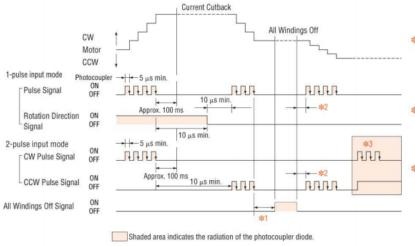
Note: 10 µs or more is the standard interval time for switching from CW to CCW. Note that the interval time varies greatly depending on the motor and load inertia.
