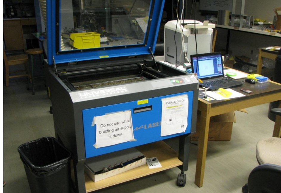
Laser Cutter/Engraver – cardboard, wood, plastics.
